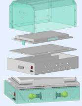
THE OBJECTIVE IS TO KEEP THE TEMPERATURE AROUND 33 - 35 O C, PREVENT THE OVERHEAT. SAFETY IS THE MAIN PRIORITY AFTER ALL. BASICALLY, OUR INCUBATOR UTILIZES NATURAL CIRCULATION FROM THE AIR TO WARM THE CABIN ITSELF.
